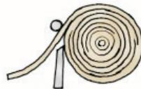
**Lathe Peeling:** The Raute Wood Lathe scans the log profile using 7 lasers, then centres the log for the most efficient recovery of material and peels the logs to a core diameter of 78mm. All round-up, waste veneer and cores are converted into chip, which is used in the manufacture of MDF. Equipment Supplier: Raute Wood.
